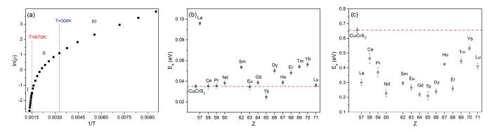
**Figure 3.** Inverse temperature dependence of electrical resistivity in logarithmic scale for initial CuCrS<sub>2</sub>-matrix (**a**) and activation energy values for doped CuCr<sub>0.99</sub>Ln<sub>0.01</sub>S<sub>2</sub> (Ln = La. . .Lu) disulfides at temperatures below 300 K (**b**) and in a high-temperature range (**c**).
