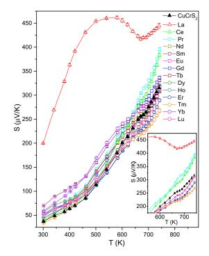
**Figure 1.** Seebeck coefficient temperature dependencies for initial CuCrS<sub>2</sub>-matrix and doped CuCr<sub>0.99</sub>Ln<sub>0.01</sub>S<sub>2</sub> (Ln = La...Lu) disulfides. Inset: The enlarged region of the S(T) within a temperature range ~100 K below and ~50 K above the ODT.
