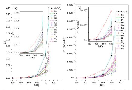
**Figure 6.** Thermoelectric figure of merit (**a**) and power factor (**b**) temperature dependencies for initial  $CuCrS_2$ -matrix and doped  $CuCr_{0.99}Ln_{0.01}S_2$  (Ln = La...Lu) disulfides.
