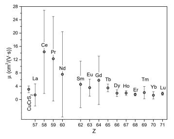
**Figure 4.** Hall mobility for initial CuCrS<sub>2</sub>-matrix and doped CuCr<sub>0.99</sub>Ln<sub>0.01</sub>S<sub>2</sub> (Ln = La...Lu) disulfides at 300 K.
