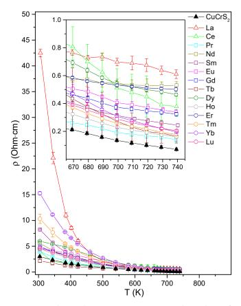
**Figure 2.** Electrical resistivity temperature dependence for initial CuCrS<sub>2</sub>-matrix and doped CuCr<sub>0.99</sub>Ln<sub>0.01</sub>S<sub>2</sub> (Ln = La. . . Lu) disulfides.
