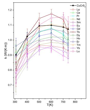
**Figure 5.** Thermal conductivity temperature dependencies for initial CuCrS<sub>2</sub>-matrix and doped CuCr<sub>0.99</sub>Ln<sub>0.01</sub>S<sub>2</sub> (Ln = La. . . Lu) disulfides.
