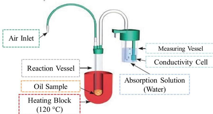
**Figure 1.** Principle of the Rancimat method.
