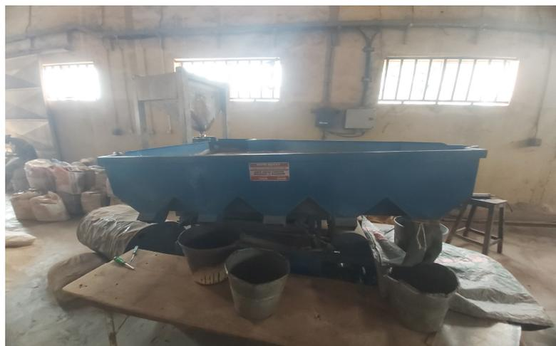
**Figure 5.** Pneumatic air-floating separator (source: National Metallurgical Development Centre (NMDC), Jos, Nigeria).
