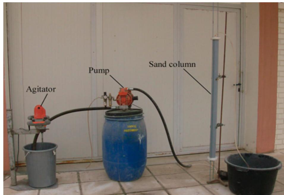
**Figure 2.** Laboratory simulation of the grouting procedure.
