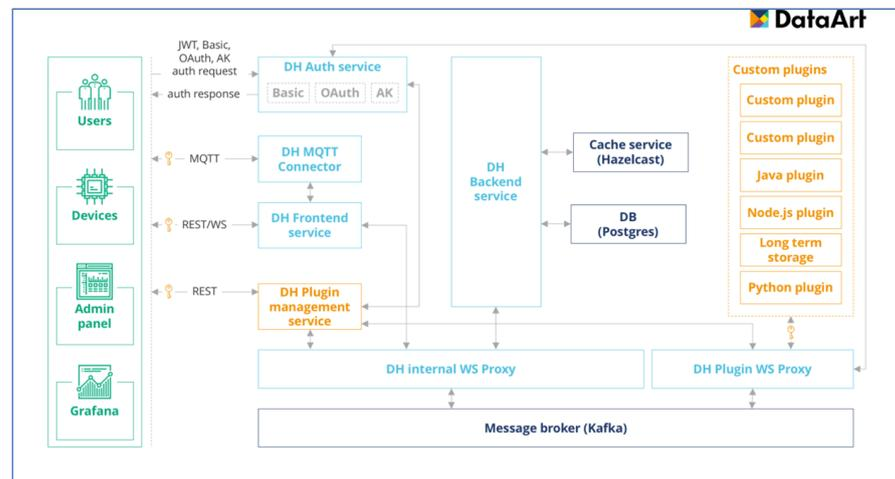
Figure 6. DeviceHive microservices architecture [64].
