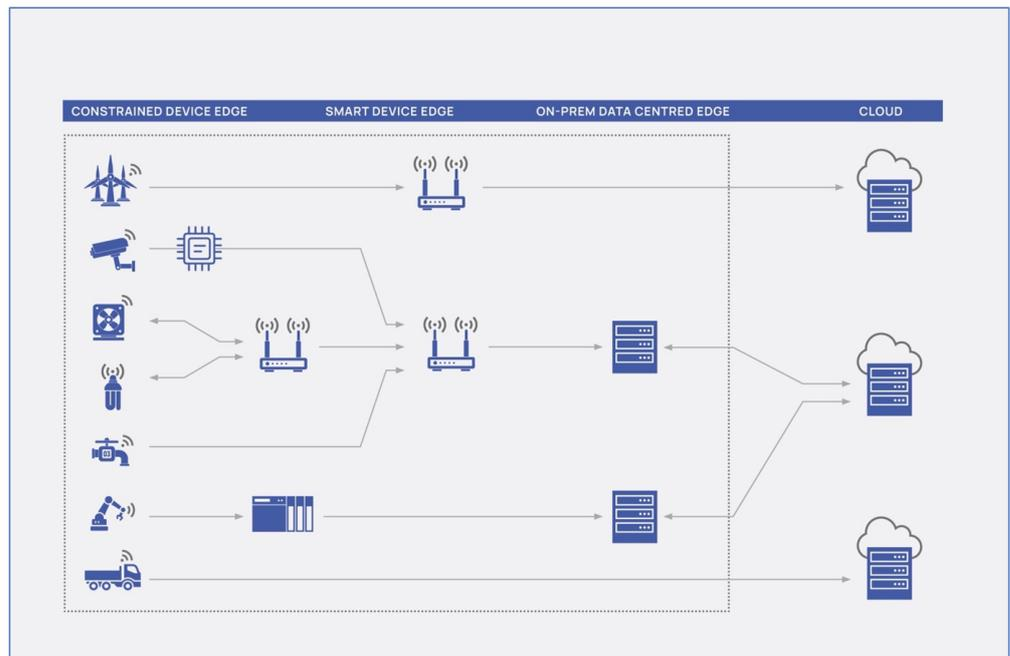
Figure 11. Edgex foundry project scope [5].
