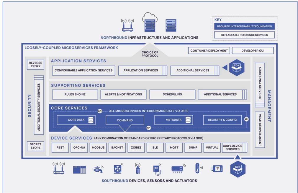
Figure 10. EdgeX platform architecture [5].
