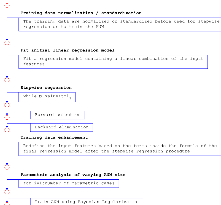
Figure 4. Workflow for estimating the optimum hidden layer size of ANNs for a given training dataset.
