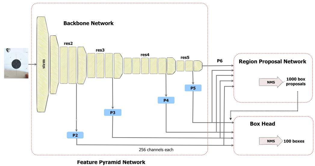
**Figure 7.** The architecture of Detectron2.
