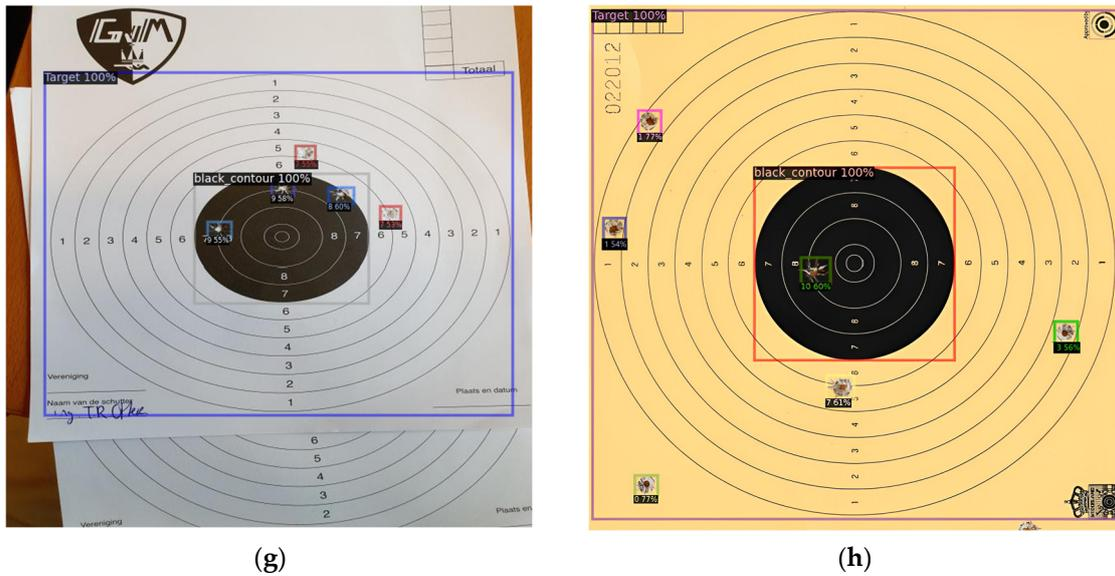
**Figure 9.** Results of bullet hole detection by detectron2 models: (a) performance of faster RCNN-101 on test image-1; (b) performance of faster RCNN-101 on test image-2; (c) performance of faster RCNN-50 on test image-1; (d) performance of faster RCNN-50 on test image-2; (e) performance of RetinaNet-50 on test image-1; (f) performance of RetinaNet-50 on test image-2; (g) performance of RetinaNet-101 on test image-1; (h) performance of RetinaNet-101 on test image-2.
