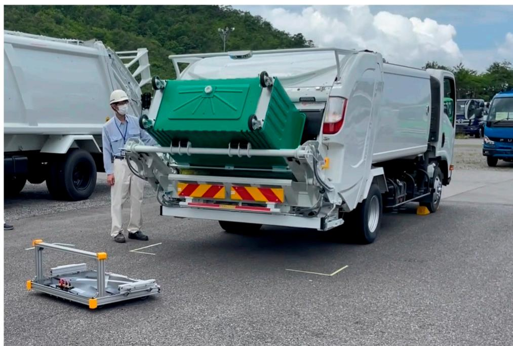
**Figure 2.** Contactless collection device that requires residents to dispose of waste in collective (green) waste containers. source: [33].
