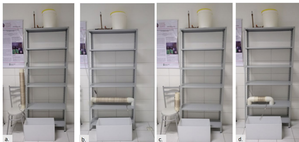
Figure 12. The alternative water clarification system with HCTF 1 in (a) vertical and (b) horizontal orientation and HCTF 2 in (c) vertical and (d) horizontal orientation. Source: Authors (2023).
