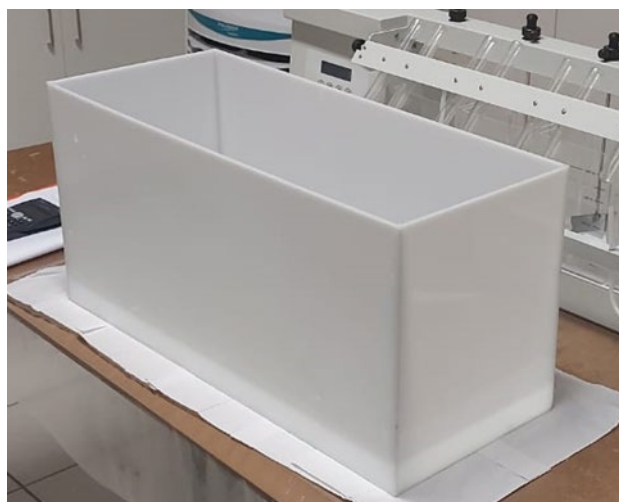
Figure 3. Decanter used in the alternative water clarification system. Source: Authors (2023).
