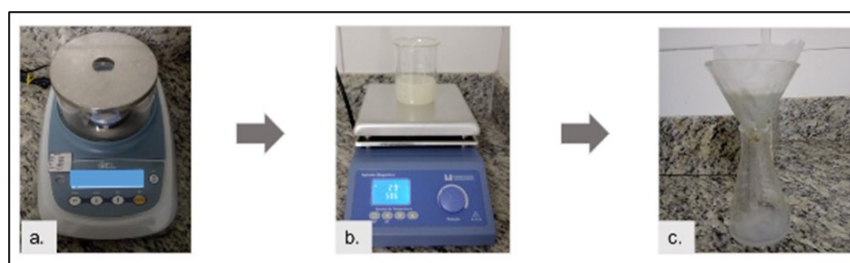
Figure 9. Coagulant solution preparation process using ground Moringa oleifera seed powder: (a) weighing, (b) stirring, and (c) filtering. Source: Authors (2023).
