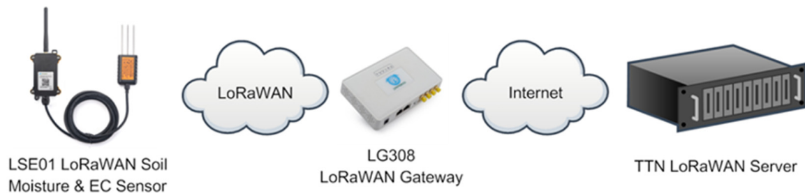
Figure 2. LoRaWAN used for continuous soil moisture data collection [34].
