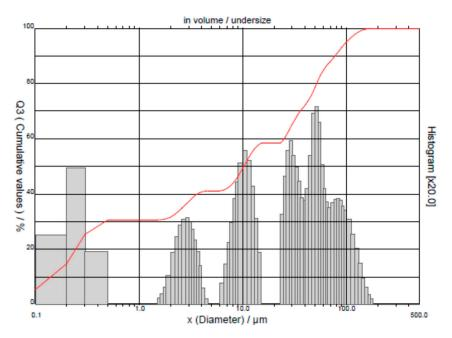
**Figure 5.** Particle size distribution of solids in the form of dust from the gasification technology (Note: The part on the left side of figure are diameters of particles distributions cumulative values in logarithmic scale.) [28].
