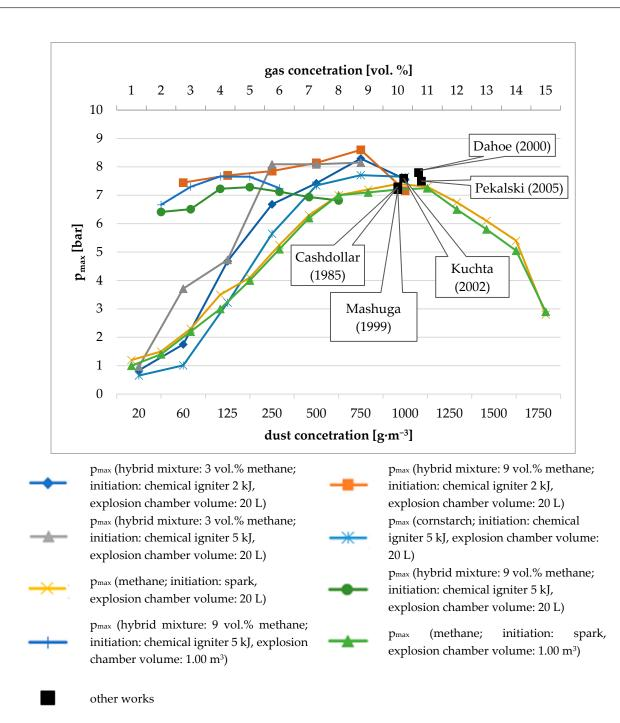
**Figure 11.** Comparison of the maximum explosion pressure of methane, cornstarch and their hybrid mixture [10].
