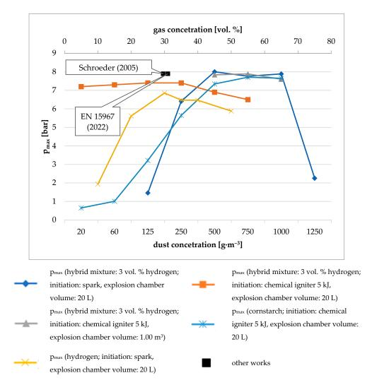
**Figure 9.** Comparison of the maximum explosion pressure of hydrogen, cornstarch and their hybrid mixture [30,33].
