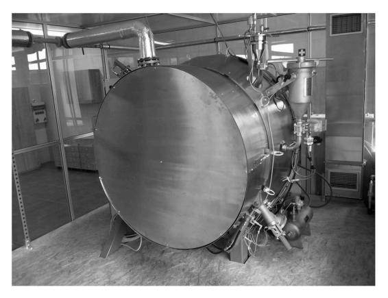
Figure 2. Illustrative picture of the explosion chamber CA 1M3 [21].
