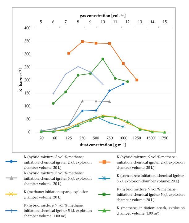
Figure 12. Comparison of the cubic constant of methane, corn starch and their hybrid mixture.
