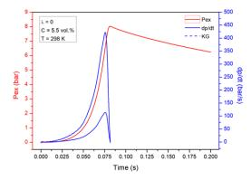
**Figure 1.** Example of primary pressure records for H<sub>2</sub>.
