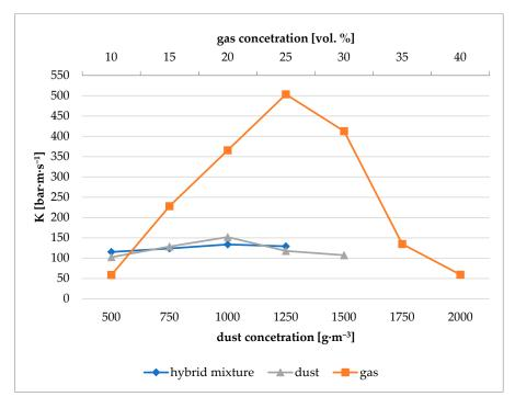
Figure 8. Comparison of the cubic constant of syngas, gasification dust and their hybrid mixture.
