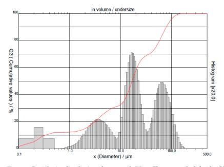
**Figure 4.** Particle size distribution of corn starch (Note: The part on the left side of figure are diameters of particles distributions cumulative values in logarithmic scale.) [27].
