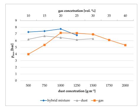
**Figure 7.** Comparison of maximum explosion pressure of syngas, gasification dust and their hybrid mixture.
