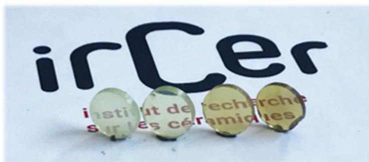
**Figure 3.** Transparent Ho:Lu<sub>2</sub>O<sub>3</sub> ceramics with various Ho<sup>3+</sup> doping rates (from the left to the right: 0.5 at.%, 1 at.%, 5 at.% and 10 at.%) sintered by SPS at 1400 °C for 15 min under 130 MPa of uniaxial pressure.
