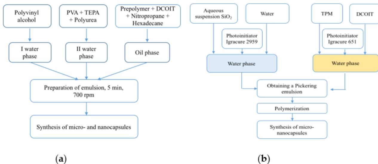
**Figure 4.** A scheme for the synthesis of microcapsules loaded with the biocide DCOIT (a) for microcapsules with a polyurea shell and DCOIT biocide in the core and (b) for microcapsules with a shell made of silicon dioxide nanoparticles and a core of polymethacrylate containing DCOIT.
