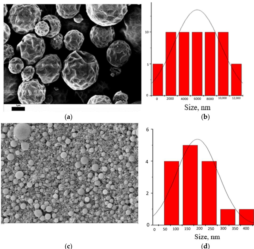
**Figure 6.** SEM micrographs and particle size distribution curves: (a,b) microcapsules with a shell made of silicon dioxide nanoparticles and a core of polymethacrylate containing DCOIT [40]; (c,d) microcapsules with a polyurea shell with DCOIT biocide in the core [96].
