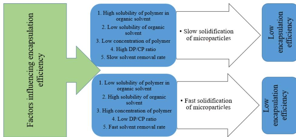
**Figure 3.** Factors influencing encapsulation efficiency.
