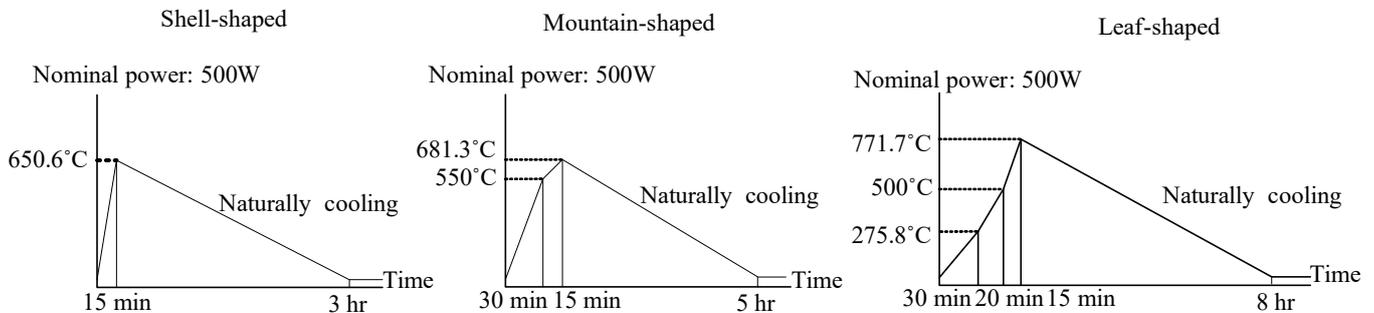
**Figure 7.** Casting glass firing temperature curves.
