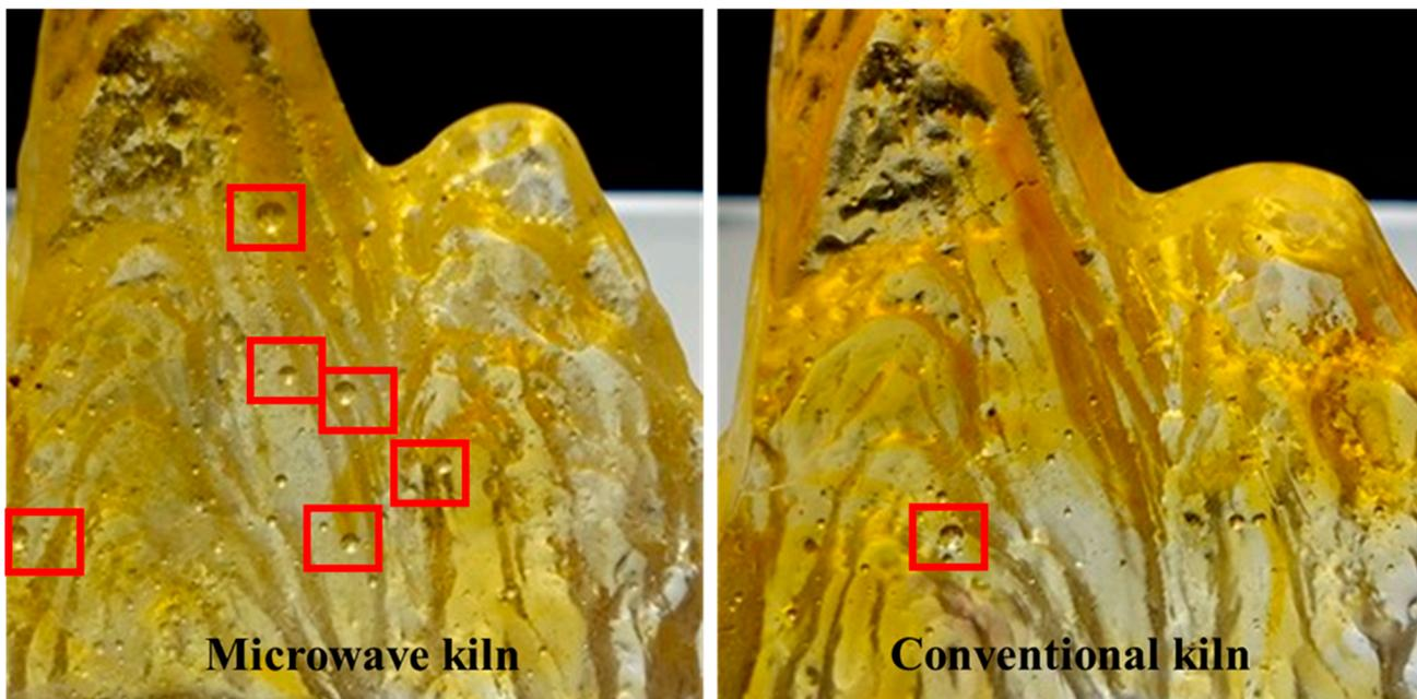
**Figure 9.** Comparison of the number of air bubbles in 3D glass artworks fired in different kilns.
