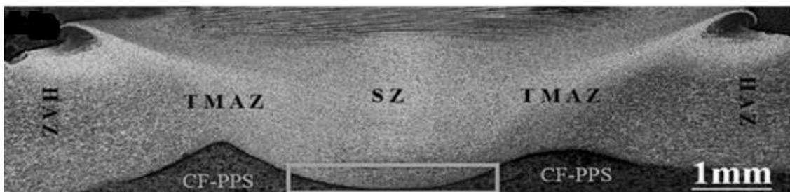
Figure 17. Refill FFSW aluminum–carbon fiber thermoplastic composite weld joint morphology [138].
