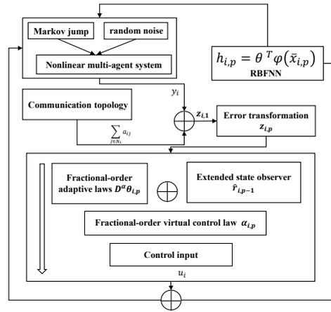
Figure 1. Block diagram of the system controller design.
