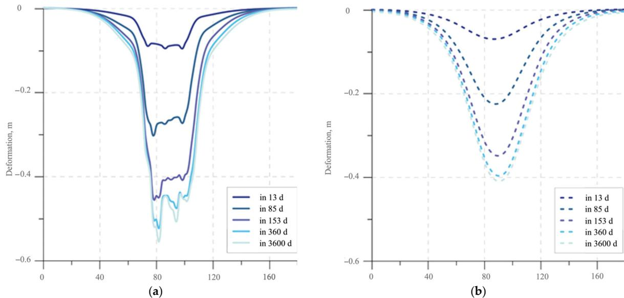
**Figure 10.** Vertical deformation. (a) Deformation 15 m above the roof; (b) Deformation 50 m above the roof.
