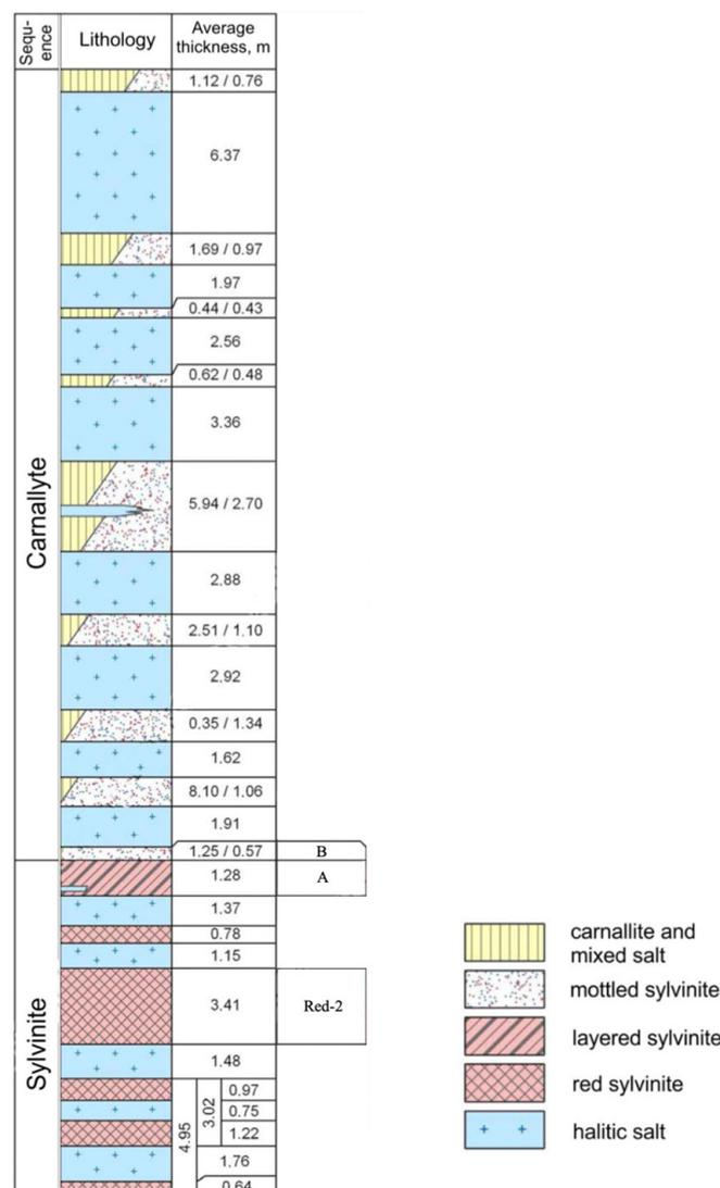
Figure 2. Stratigraphy of the Verkhnekamsk potash deposit.
