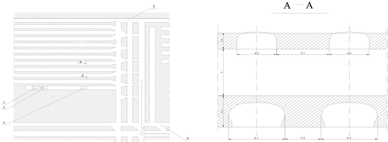
**Figure 3.** Mining method at the Verkhnekamsk potash deposit. 1—combine; 2—bunker reloader; 3—self-propelled car; 4—transport road; and 5—ventilation drift.
