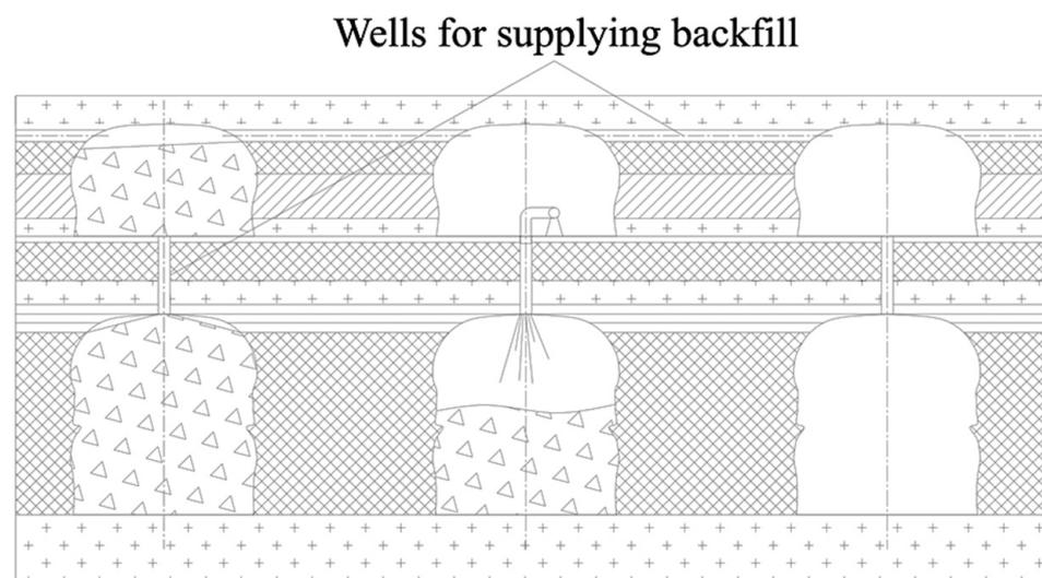
**Figure 8.** Scheme of feeding of backfill into the rooms.
