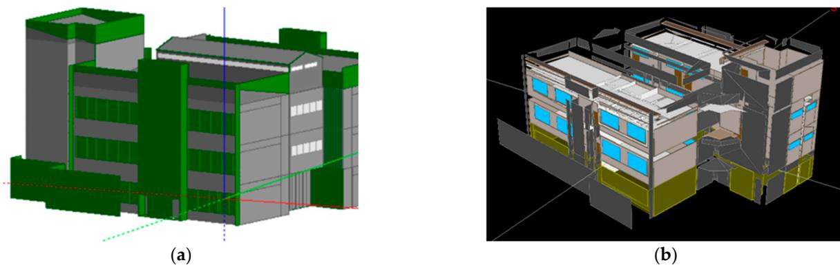
**Figure 6.** Failures on detailed geometry transfer from Building 5T in different BES software: (a) DesignBuilder, (b) eQUEST.
