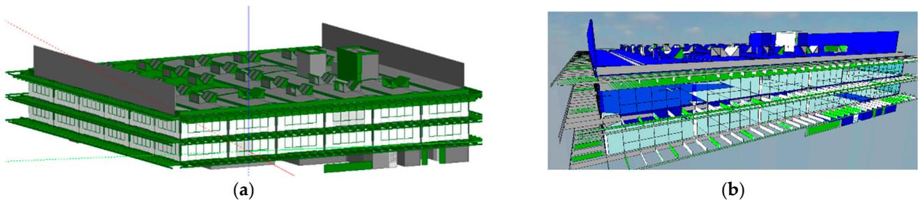
**Figure 5.** Failures on detailed geometry transfer from the library in different BES software: (a) DesignBuilder, (b) IES-VE.
