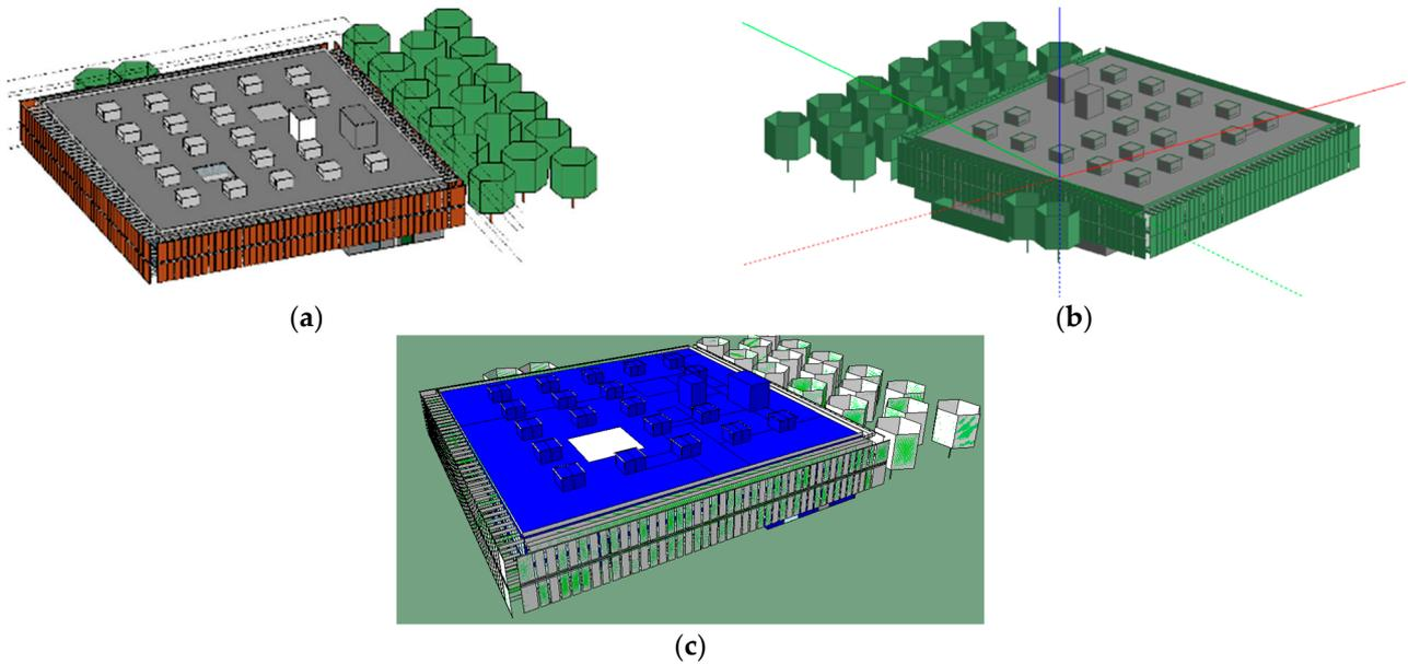
**Figure 7.** Simplified geometry exportation from the library to different BES software: (a) Revit, (b) DesignBuilder, and (c) IES-VE.
