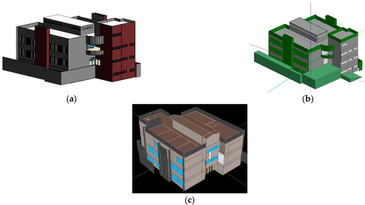
**Figure 8.** Simplified geometry exportation from Building 5T to different BES software: (a) Revit, (b) DesignBuilder, and (c) eQUEST.
