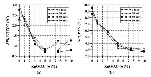
Figure 5. Evolution of SPI with ZnO/AC content and MT. (a) RTFOT, and (b) PAV.
