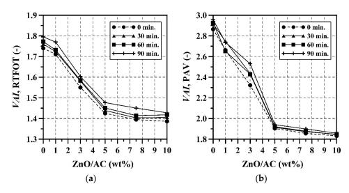
Figure 6. Evolution of VAI with ZnO/AC content and MT. (a) RTFOT, and (b) PAV.
