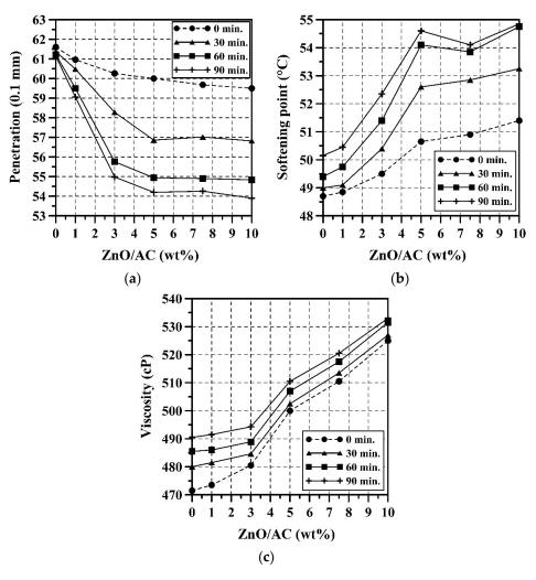
**Figure 3.** Evolution of (**a**) penetration, (**b**) softening point, and (**c**) viscosity with ZnO/AC content and MT.
