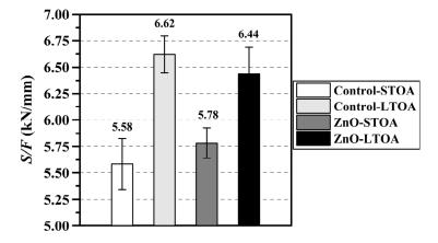
Figure 8. S/F ratio—Control and modified samples under STOA and LTOA condition.
