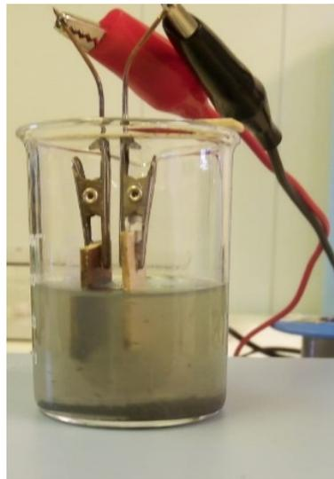
Figure 21. Picture at the end of the electrophoretic deposition method.
