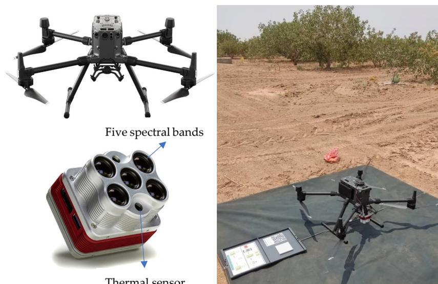
**Figure 2.** DJI Matrice 300 RTK drone (DJI, Frankfurt, Germany) and Altum MicaSense sensor used for image collection.
