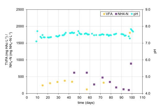
Figure 3. Characteristics of the digestate's liquid phase during the fermentation test.
