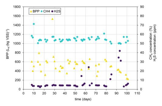
Figure 4. BPP as well as CH<sub>4</sub> and H<sub>2</sub>S concentration during the fermentation test.
