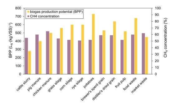
**Figure 1.** Biogas production potential (BPP) and average CH<sub>4</sub> concentration of substrates commonly used in anaerobic digestion. Data compiled from [9–12].
