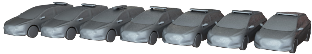
Figure 7. A rendered image of the positional changes to the standard lightbar on the Hyundai i40.
