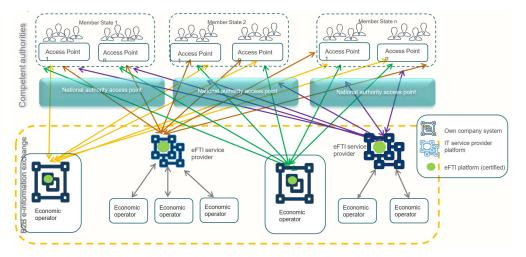
Figure 1. eFTI exchange environment—potential implementation architecture [6].
