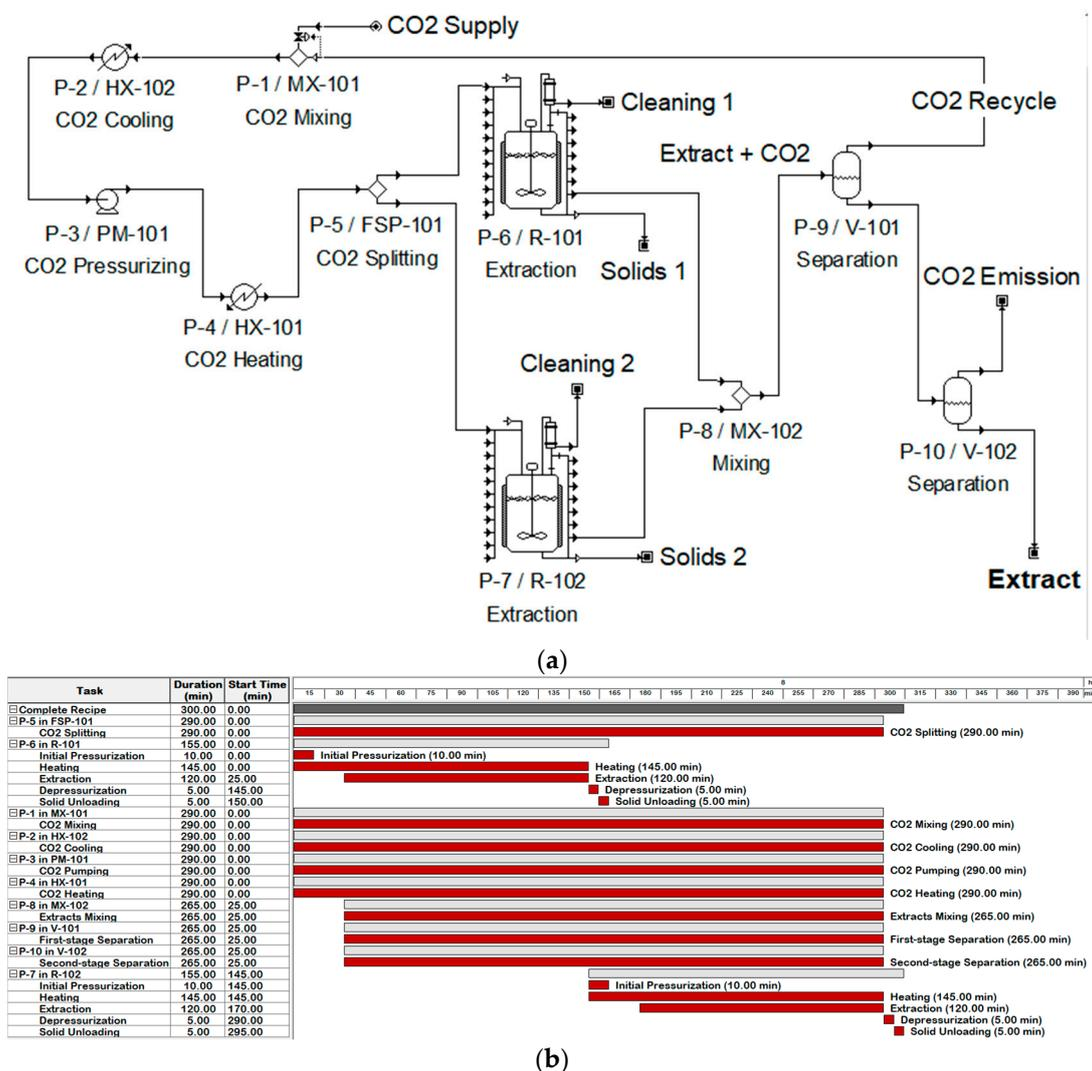
Figure 3. (a) Process flowsheet and (b) a Gantt chart for an extraction time of 120 min.
