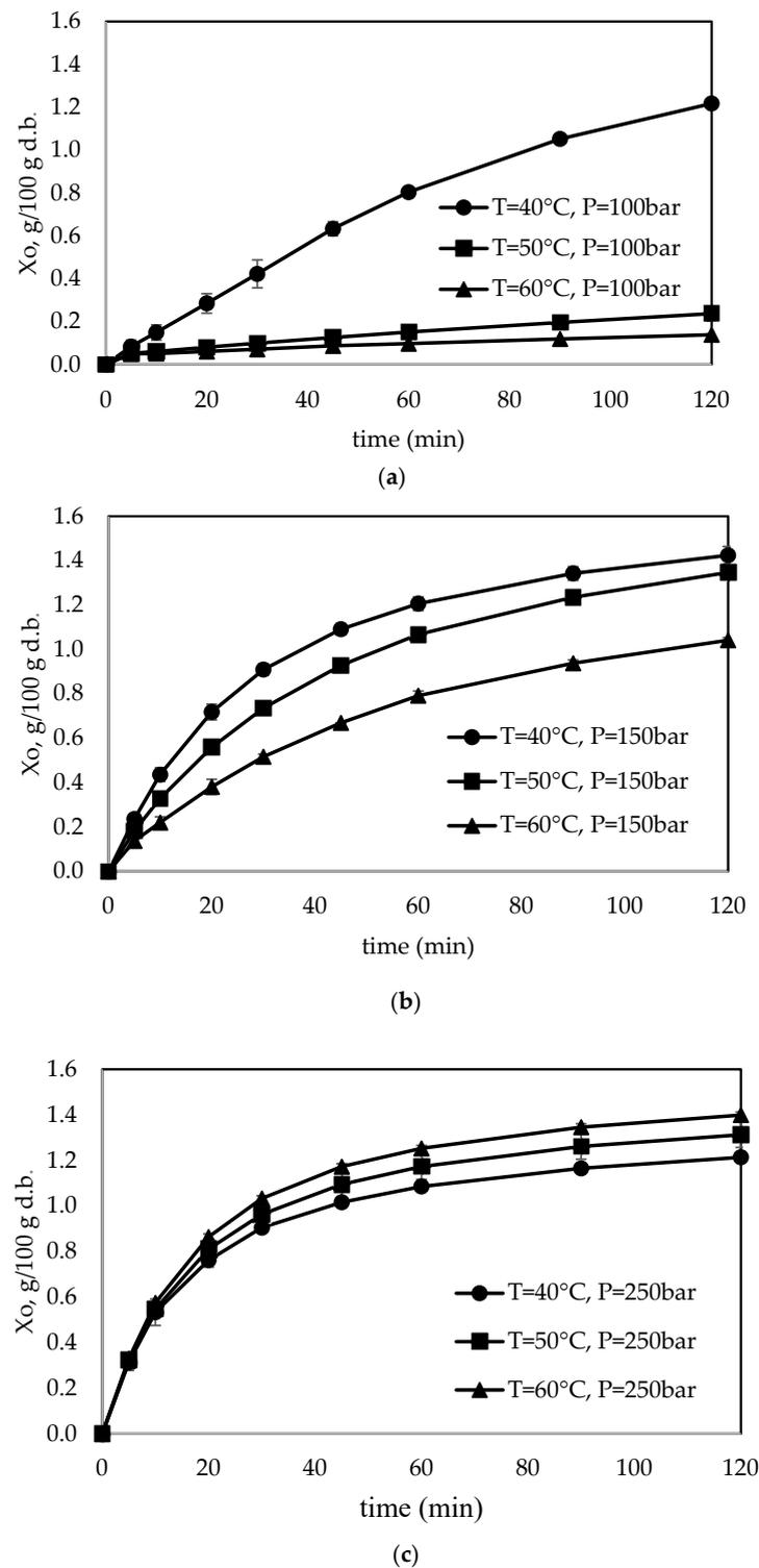
**Figure 4.** Overall extraction curve (OEC) for the studied conditions: (a) 100 bar, (b) 150 bar, and (c) 250 bar.
