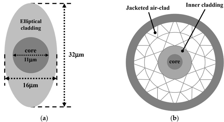
**Figure 2.** Schematic cross-sections of the elliptical inner cladding fiber (a) and JAC fiber (b).
