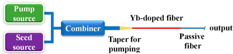
Figure 5. Schematic experimental setup of Yb-doped fiber amplifier in Ref. [35].
