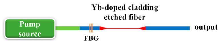
Figure 6. Schematic experimental setup of Yb-doped fiber laser in Ref. [36].
