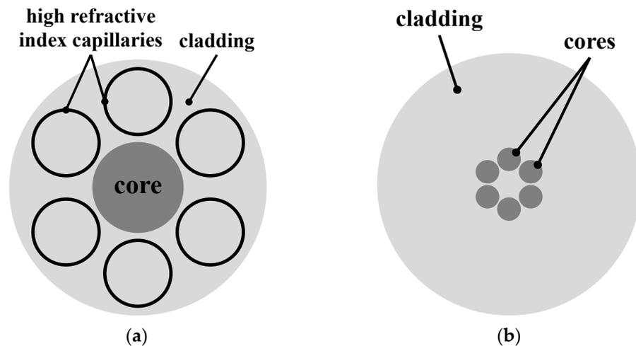
**Figure 8.** Schematic cross-sections of the YbARF [56] (a), and the Yb-doped 6-core fiber [57] (b).
