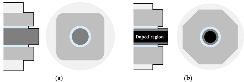
**Figure 7.** Schematic refractive index profiles and cross-sections of the W-profile Yb-doped fiber in Ref. [43] (a), and the confined Yb-doped fiber in Ref. [44] (b).
