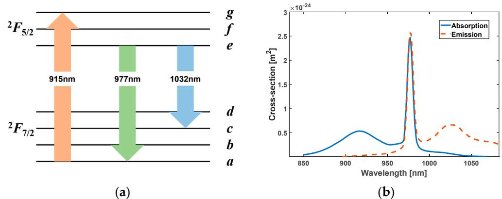
Figure 1. (a) Energy-level diagram (a-g represent different states and a represents the ground state), and (b) typical absorption and emission cross-sections of Yb-ions.
