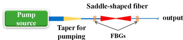
Figure 4. Schematic experimental setup of saddle-shaped Yb-doped fiber laser near 980 nm.
