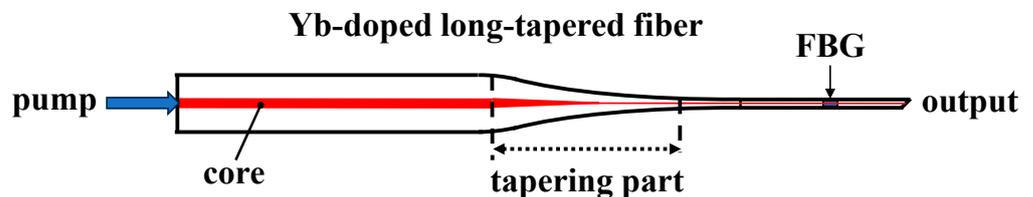
**Figure 3.** Schematic experimental setup of the long-tapered fiber laser in Ref. [33].
