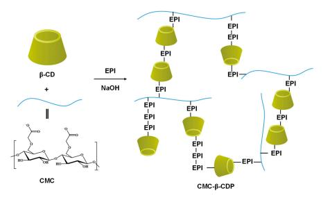
**Figure 5.** Synthesis route of CMC–*β*–CD polymer [51].
