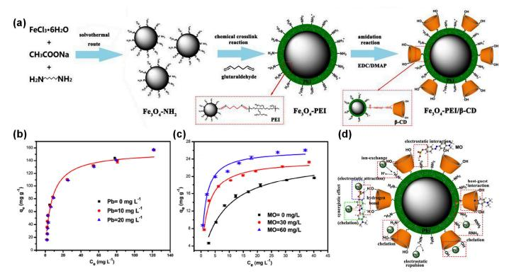
**Figure 15.** (a) Synthesis route of  $Fe_3O_4$ –PEI/ $\beta$ –CD composite; adsorption isotherms of MO (b) and Pb<sup>2+</sup> (c) by  $Fe_3O_4$ –PEI/ $\beta$ –CD in the presence of different concentrations of Pb<sup>2+</sup> or MO; (d) proposed mechanisms for the simultaneous capture of MO and Pb<sup>2+</sup> by  $Fe_3O_4$ –PEI/ $\beta$ –CD [68].
