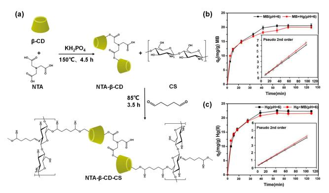
**Figure 21.** (a) Synthesis of NTA– $\beta$ –CD–CS; the effect of contact time on the adsorption of (b) Hg<sup>2+</sup> and (c) MB by NTA– $\beta$ –CD–CS in mono and binary systems [76].
