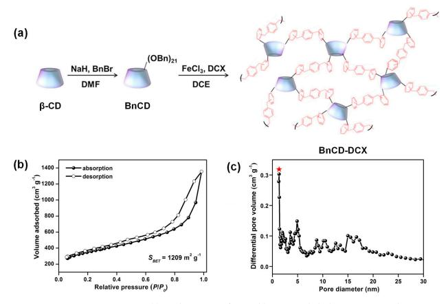
**Figure 11.** (a) Synthesis route of a novel hyper–crosslinked  $\beta$ –CD porous polymer BnCD–DCX; (b) N<sub>2</sub> adsorption–desorption isotherm of BnCD–DCX measured at 77K; (c) the aperture fraction of BnCD–DCX calculated by NDLFT [55].
