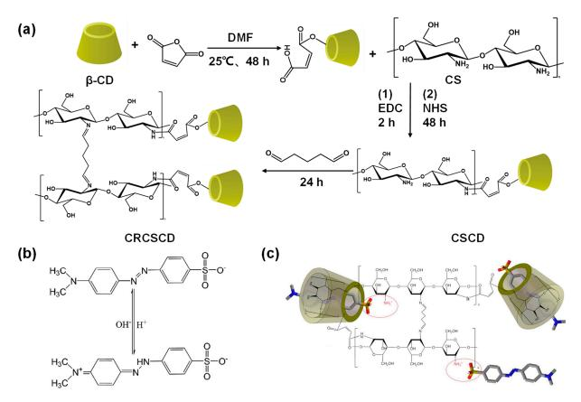
**Figure 20.** (a) Synthesis of CRCSCD; (b) the structure of the MO molecule; (c) adsorption mechanism of MO adsorbed by CRCSCD [75].
