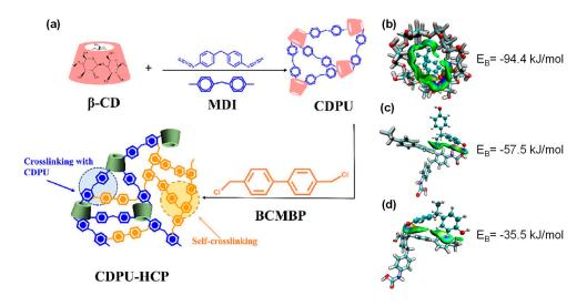
**Figure 6.** (a) Synthesis route of CDPU–HCP; optimized configurations of BPA adsorbed on three active adsorption sites of CDPU–HCP: BPA on (b)  $\beta$ –CD cavity, (c) urethane bond, and (d) aromatic ring of CDPU–HCP and their corresponding binding energies. Illustration of the dispersed IGM isosurface domains (0.003 a.u.) for these configurations [53].
