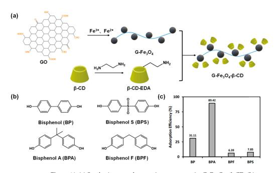
**Figure 14.** (a) Synthesis route of magnetic nanocomposite G–Fe<sub>3</sub>O<sub>4</sub>– $\beta$ –CD; (b) structure of bisphenol analogues; (c) the adsorption selectivity of nanocomposites to BPA [67].
