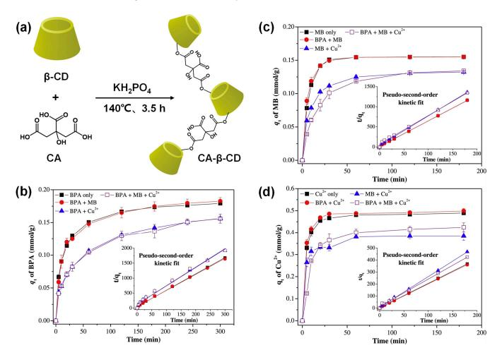
**Figure 7.** (a) Synthesis route of CA– $\beta$ –CD, influence of contact time on the adsorption of (b) BPA, (c) MB, and (d) Cu<sup>2+</sup> by CA– $\beta$ –CD in single–component or multi–component systems from aqueous solutions [40].
