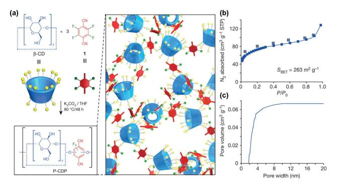
**Figure 10.** (a) Synthesis route of P–CDP; (b) N<sub>2</sub> adsorption (blue box) and desorption (gray box) isotherms of P–CDP; (c) cumulative pore volume of P–CDP obtained by NLDFT analysis [44].
