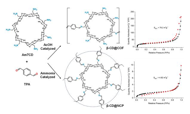
**Figure 12.**  $\beta$ -CD@COF and  $\beta$ -CD@NCP prepared under different catalytic conditions and their respective N<sub>2</sub> adsorption (black squares) and desorption (red squares) isotherms measured at 77 K [61].
