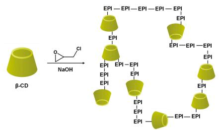
**Figure 3.** Crosslinking reaction of  $\beta$ -CD with epichlorohydrin [51].
