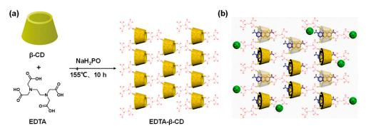
**Figure 9.** (a) Synthesis route of EDTA– $\beta$ –CD; (b) adsorption mechanism of Cu<sup>2+</sup> and dyes by EDTA– $\beta$ –CD [42].
