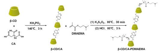
Figure 8. Synthesis route of the amphoteric  $\beta$ -CD/CA-PDMAEMA [57].
