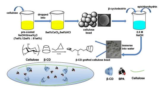
**Figure 22.** Preparation of  $\beta$ -CD-grafted cellulose beads for the removal of BPA via host-guest interactions [77].
