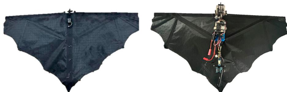
**Figure 9.** Bat-like ornithopter prototype.
