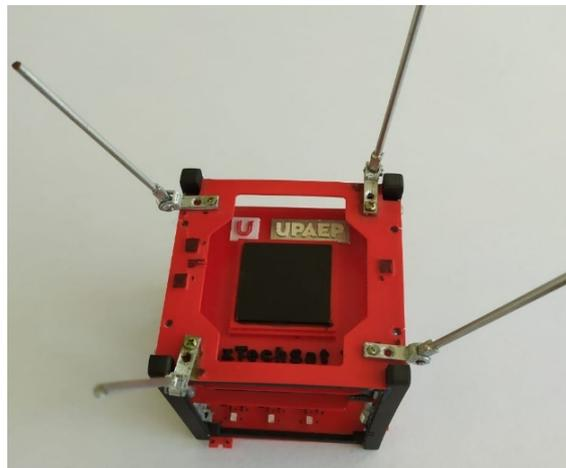
**Figure 6.** 3D printed version of AztechSat-1.
