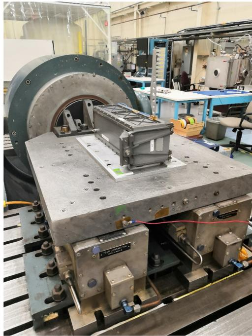
**Figure 14.** Vibration test setup.
