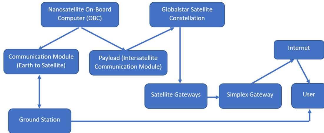
**Figure 2.** AztechSat-1 communication block diagram.
