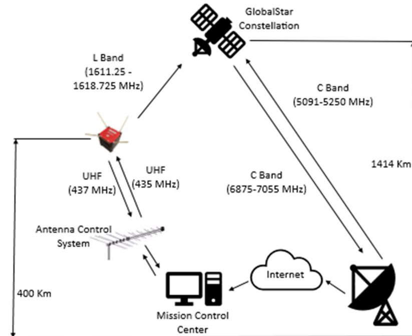
**Figure 1.** AztechSat-1 mission operation diagram.
