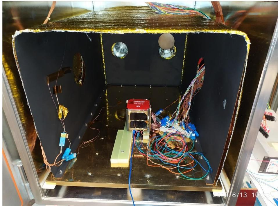
**Figure 16.** Thermal vacuum test setup.
