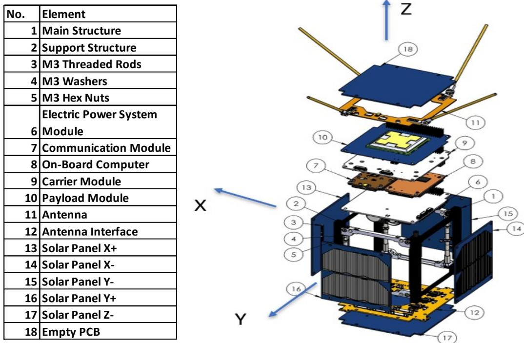
Figure 5. AztechSat-1 design obtained from sprints.
