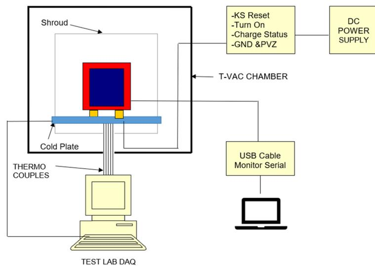
**Figure 9.** Temperature data acquisition system for AztechSat-1.
