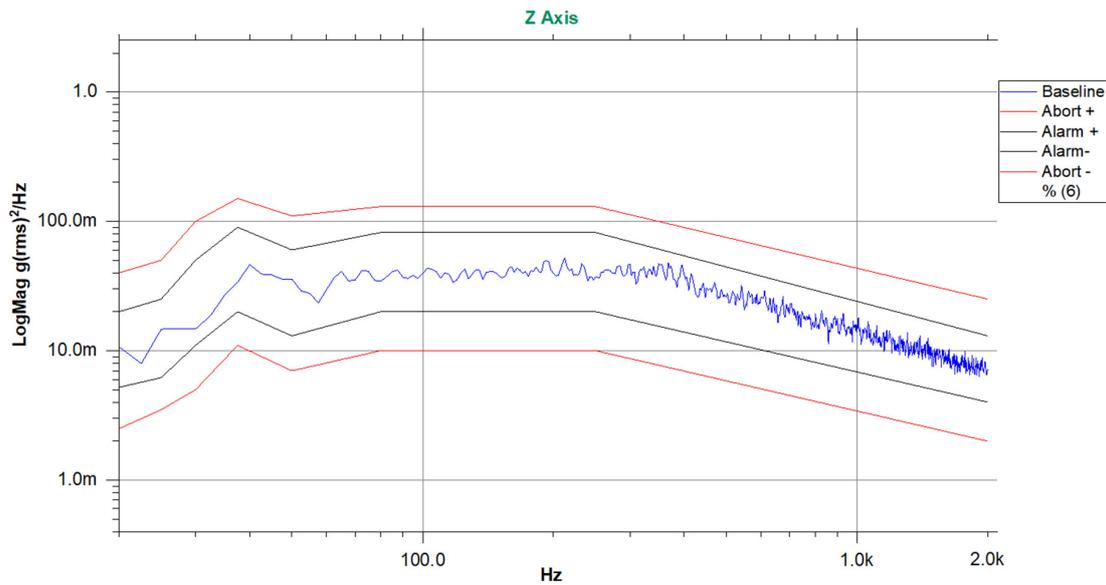
Figure 12. Random vibration test (PSD response for the Z axis).
