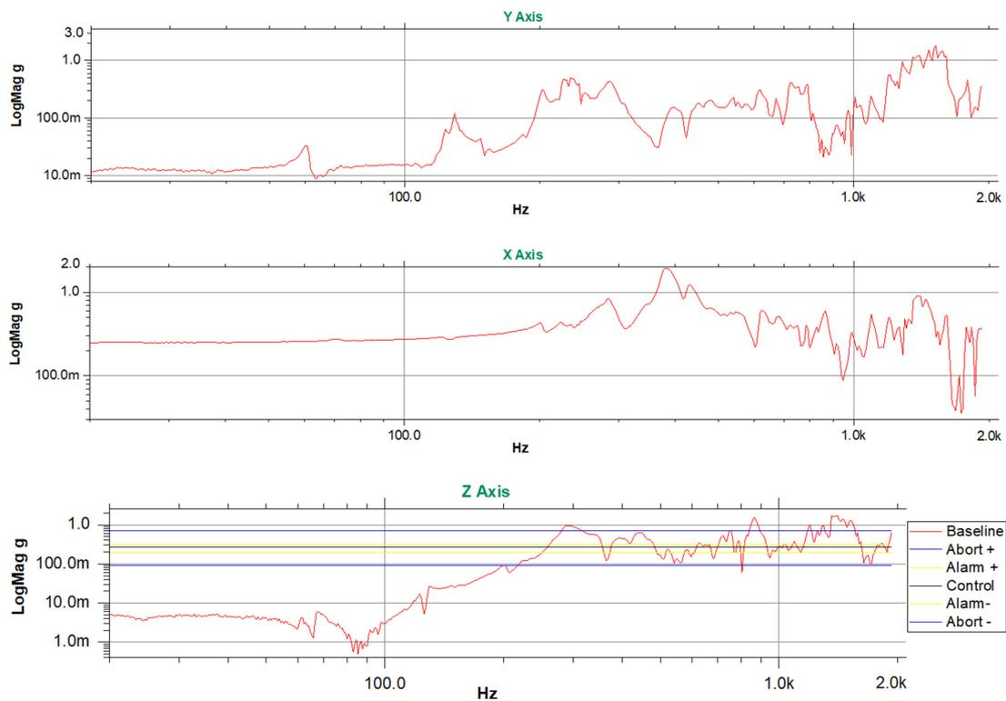
Figure 13. Sine sweep vibration test after the random vibration test.
