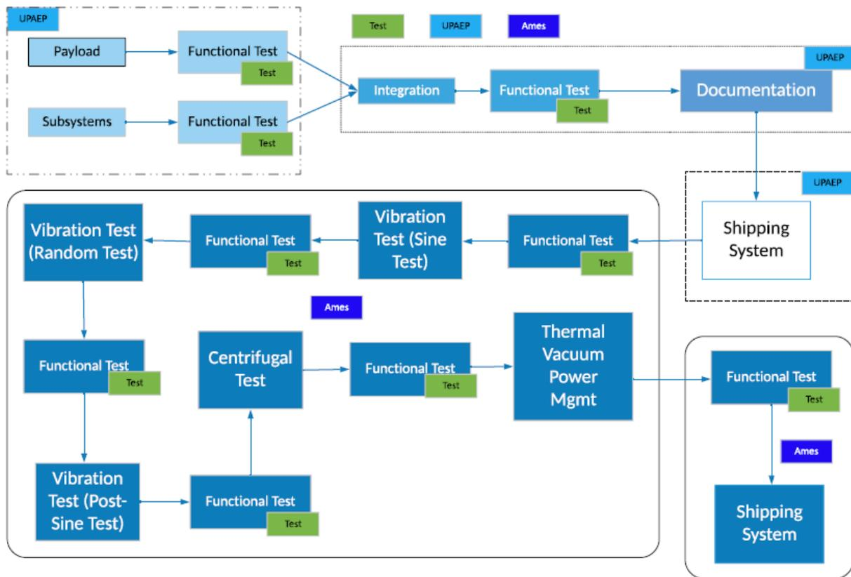
Figure 8. Testing and integration flow diagram.
