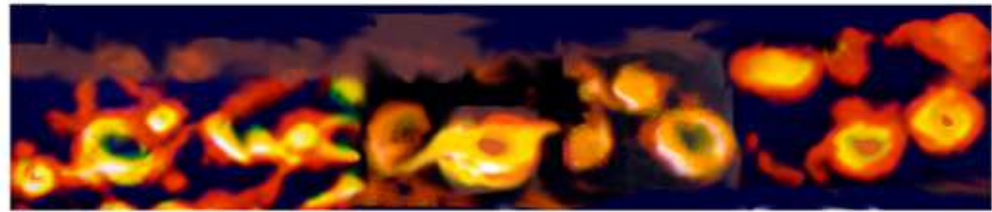
Figure 8. Breakdown of 1D loop chain into a set of open loops and vortex rings on Co-coated steel target. Vortex rings after breakdown do not move much from the former positions in the string.
