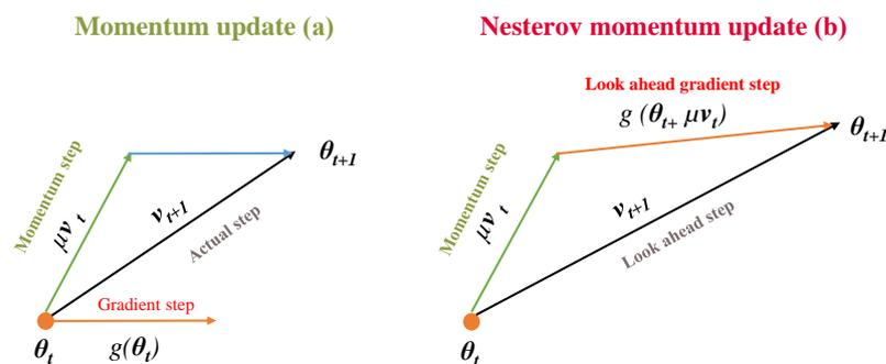
**Figure 5.** In section (a), standard gradient update; in (b), Nesterov’s momentum achieves stronger convergence by applying the velocity ( $v_t$ ) to the parameters to compute interim parameters ( $\theta = \theta_t + \mu v_t$ ), where  $\mu$  is the decay rate. These interim parameters are then used to compute the gradient, called a “look-ahead” gradient step or a Nesterov accelerated gradient.
