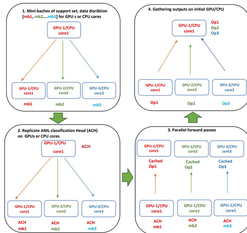
**Figure 3.** Forward pass of data using parallel computing and calculating Nesterov’s gradient. For simplicity, only three computing units are depicted.
