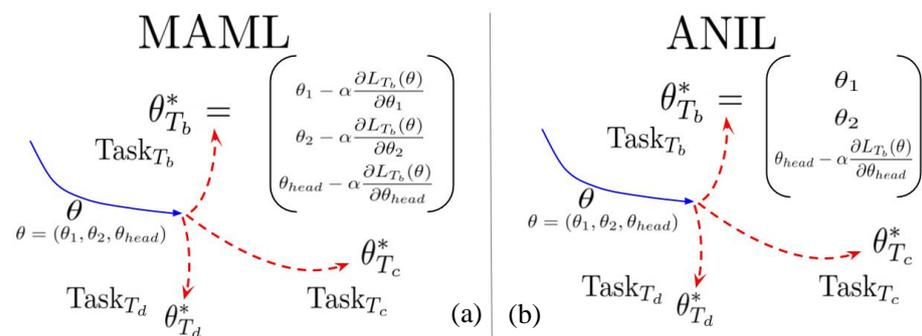
**Figure 1.** Illustration of the computations of the ANIL (b) and MAML (a) algorithms. The crucial difference between MAML (a) and ANIL (b) lies in the fact that in MAML (a), all parameters initialized with the meta-initialization from the outer loop are subject to task-specific gradient updates from the inner loop. Conversely, when training and testing ANIL (b), the inner loop solely modifies the parameters corresponding to the network head.
