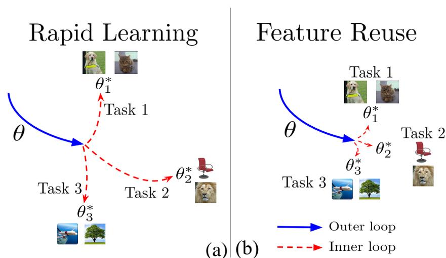
**Figure 2.** Paradigms of rapid learning (a) and feature reuse (b). In rapid learning, training in the outer loop produces parameter settings that facilitate fast learning, while updates in the inner loop result in significant task specialization. In feature reuse, the outer loop generates reusable feature-specific parameter values that do not significantly change in the inner loop.
