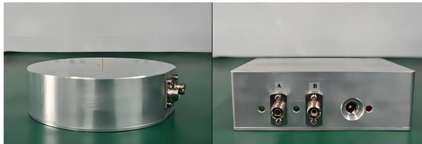
**Figure 4.** Pulsed electric-field probe and photoelectric converter.
