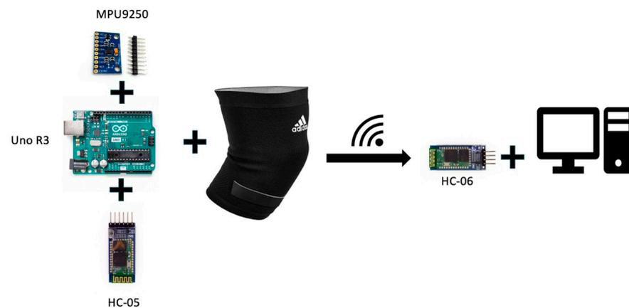
**Figure 3.** Data transmission process using the wearable module.
