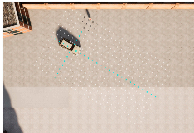
Figure 8. Occupancy grid 2D array with 30° yaw angle.
