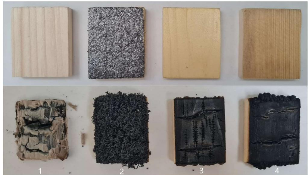
**Figure 2.** Photo documentation of samples after testing with a radiant heat source (1—untreated sample, 2—graphite with water glass, 3—Bochemit Antiflash, 4—Bochemit Pyro).
