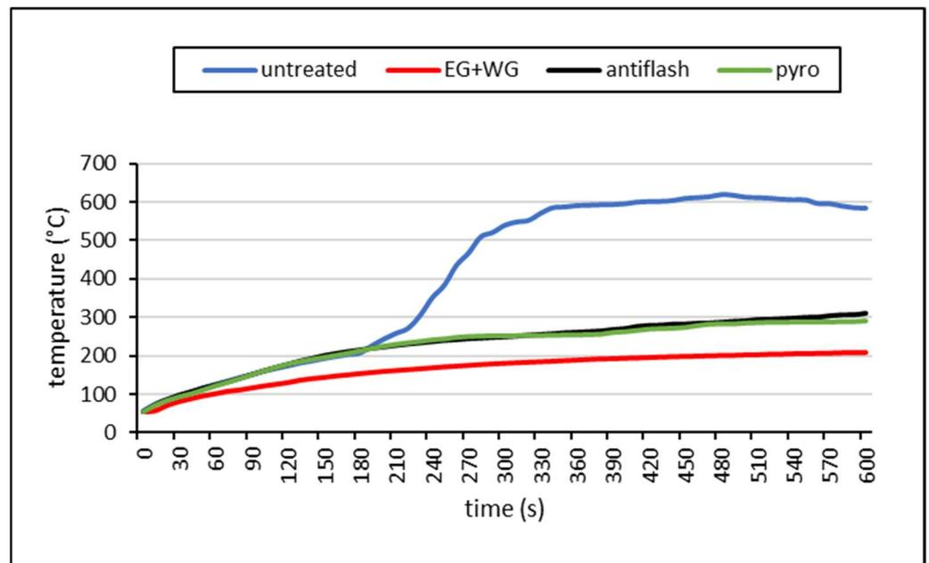
**Figure 7.** Relative temperature course of the samples at point C (untreated = reference samples, EG + WG = expandable graphite in combination with water glass, antifiash = Bochemit Antifiash, pyro = Bochemit Pyro).
