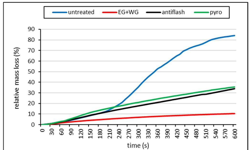
**Figure 3.** Relative mass loss of the samples during the test with a radiant heat source (untreated = reference samples, EG + WG = expandable graphite in combination with water glass, antiflash = Bochemit Antiflash, pyro = Bochemit Pyro).
