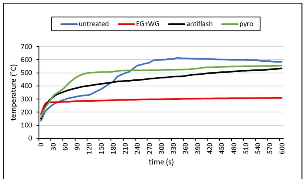
**Figure 5.** Temperature course of the samples at point A (untreated = reference samples, EG + WG = expandable graphite in combination with water glass, antifiash = Boehemit Antifiash, pyro = Boehemit Pyro).
