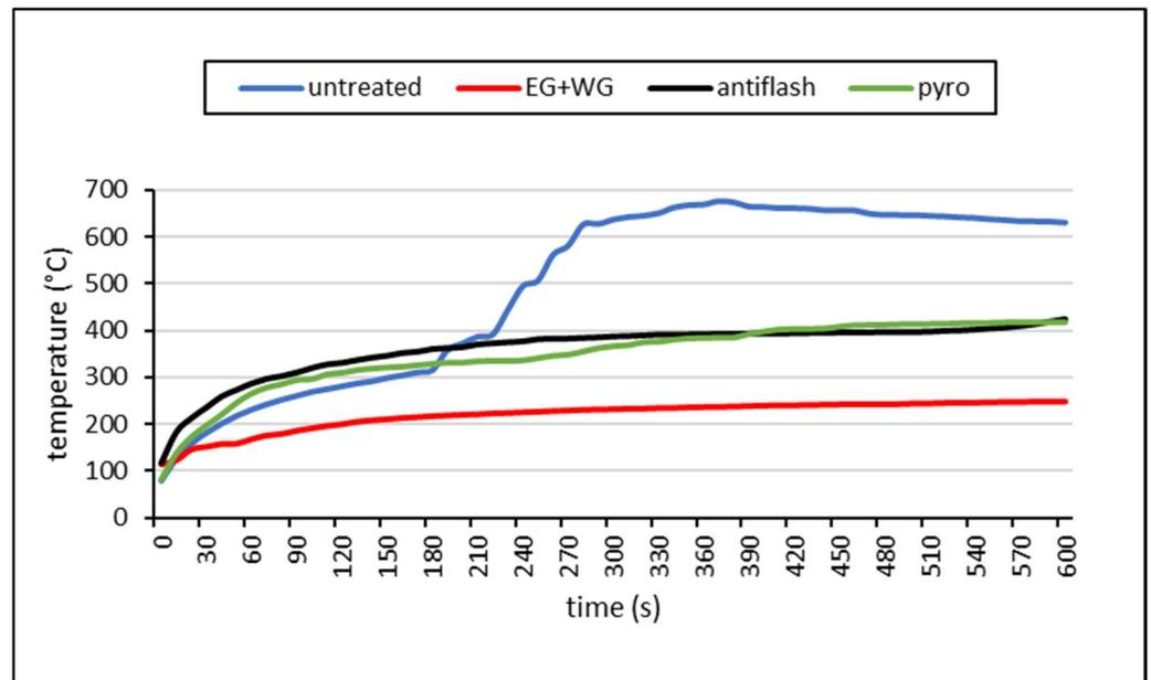
**Figure 6.** Temperature course of the samples at point B (untreated = reference samples, EG + WG = expandable graphite in combination with water glass, antifiash = Bochemit Antifiash, pyro = Bochemit Pyro).
