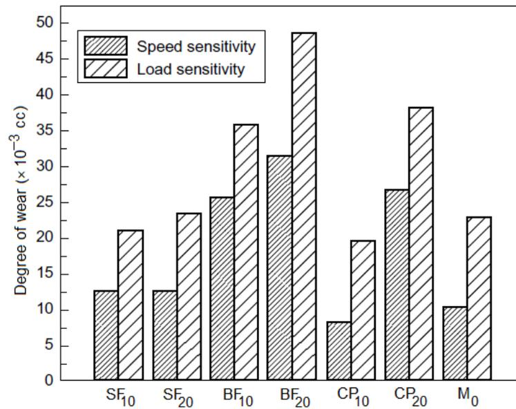
**Figure 9.** Cumulative wear behavior of composite materials based on two test methods, with speed sensitivity of 10.0, 12.5, and 15.0 m/s, respectively, load sensitivity of 2, 3, and 4 MPa, speed of 12.5 m/s, and load capacity of 3 MPa.
