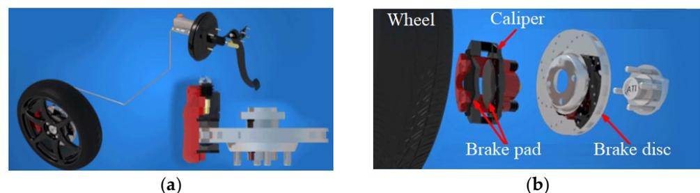
**Figure 1.** Assembly braking system (a) with the component elements (b).
