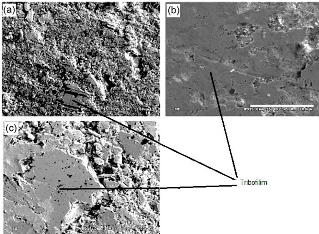
**Figure 10.** SEM images: (a) CP<sub>10</sub> (low wear and discoloration), (b) M<sub>0</sub> (high discoloration), and (c) CP<sub>20</sub> (high wear, low discoloration).
