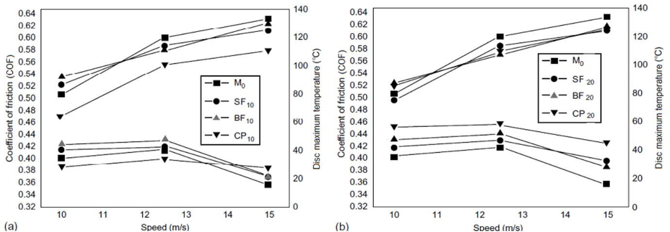
**Figure 8.** Effect of velocity on the COF of various metallic friction materials with 10 wt.% (a) and 20 wt.% (b): M<sub>0</sub>—metal-free reference material; SF—steel fiber; BF—brass fiber; CP—copper powder. Index 10 or 20 represents the metal amount in weight (10 wt.% and 20 wt.%).
