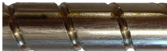
Figure 8. Example of the effect of heating on the screw worm of the gearbox.
