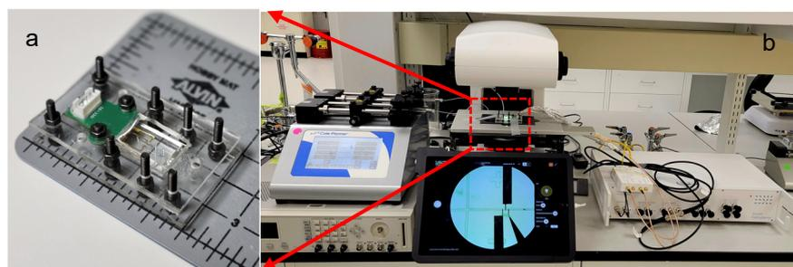
**Figure 2.** (a) The actual microfluidic chip, and (b) the measurement setup including syringe pump (left), the optical microscope (middle), and the lock in amplifier (right). The arrows show the magnified image of actual device under the optical microscope.
