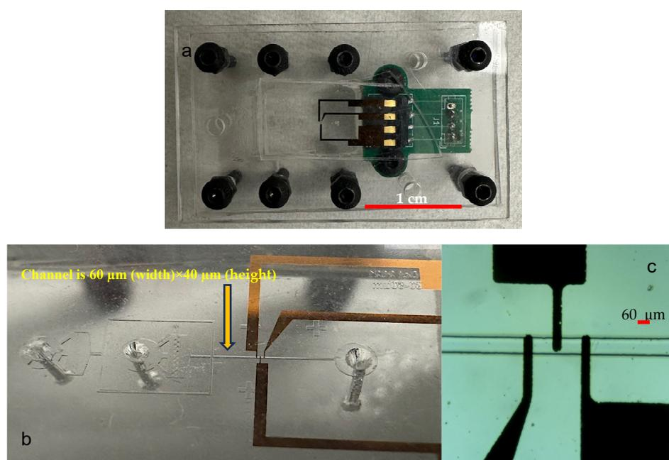
**Figure 1.** (a) The final device, (b) the dimension of the channel, and (c) the coplanar electrodes at the bottom of the microchannel.
