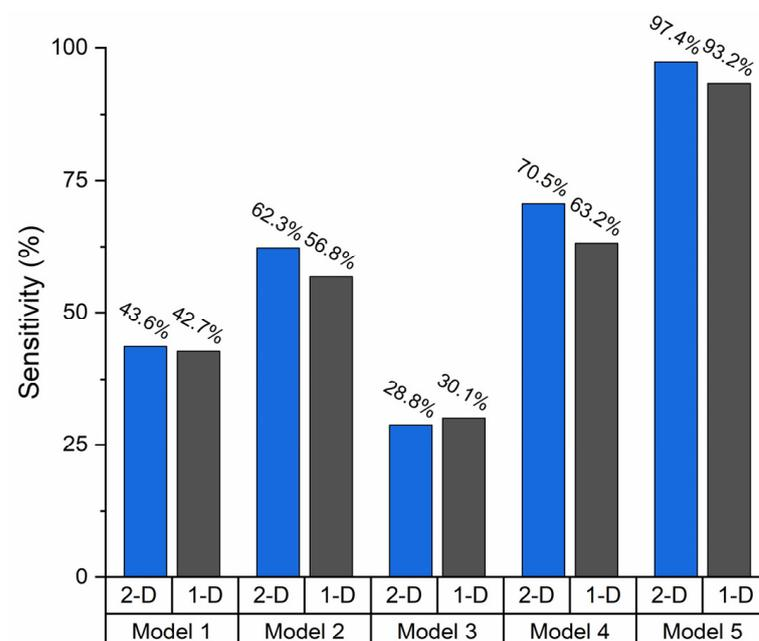
**Figure 6.** The estimated sensitivity of the device using hold-out validation for different models. The device shows poor performance in the classification of carboxyl-modified MPs, while it can successfully classify the inert ones.
