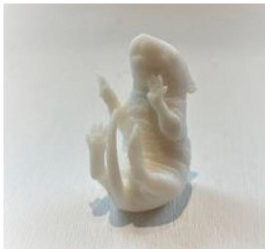
**Figure 1.** Three-dimensionally printed dummy of the P5 mouse pup. The dummy has a length of 2.7 cm, the widest part between the back and the tail is 1.8 cm, and the narrowest part between the neck and the front paw is 1.2 cm.
