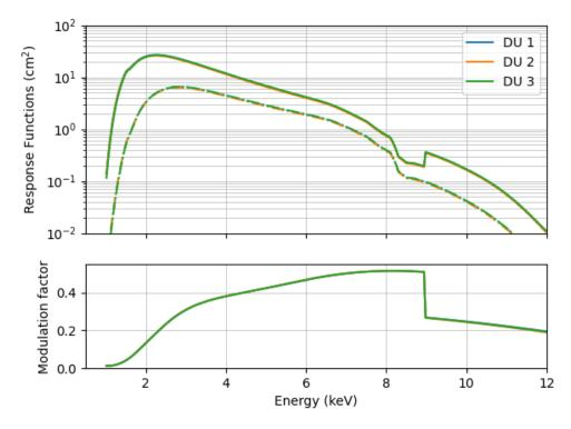
**Figure 4.** Top panel: the effective area (solid lines) and modulation response function (dash–dotted lines) of *IXPE* DU 1 (cyan), 2 (orange), and 3 (green) for a point-like, on-axis source at infinity, plotted as a function of the photon energy (notice that the curves are almost superimposed). Bottom panel: the correspondent modulation factors,  $\mu$  (note that all curves are superimposed).
