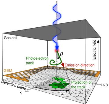
each photo-electron drifts to a gas electron multiplier (GEM), before being collected at the pixel anode.
