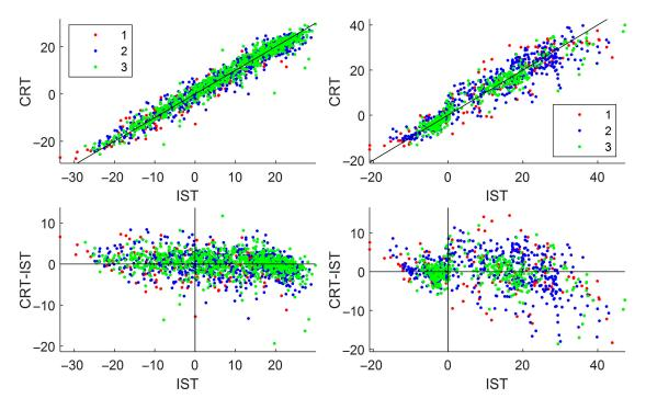
**Figure 9.** Scatter plots for CRT for air (**left**) and soil (**right**) and differences CRT–IST versus IST from 2009–2021. Lines: top panels—1:1 line, bottom panels—zero lines. 1—open sites, 2—semi-closed sites and 3—closed sites.
