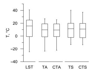
**Figure 10.** Median and quartile (25, 75%) values of LST, in situ temperatures (TA, TS) and corrected temperatures (CTA, CTS). Whiskers show 1% and 99% percentiles.
