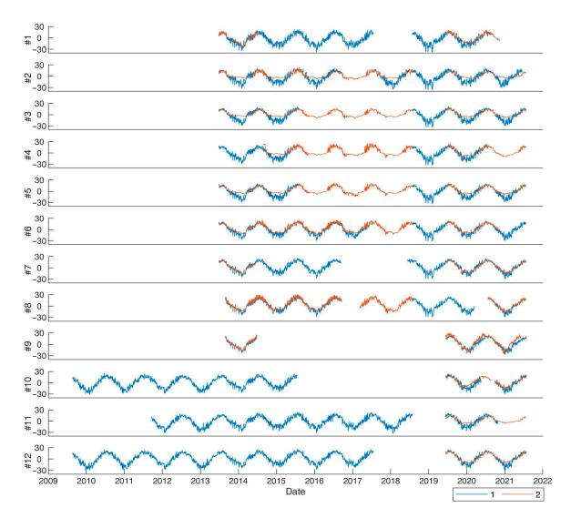
**Figure 2.** Daily average temperatures from in situ observations at 12 study sites. 1—Air IST, 2— Surface IST. Vertical axis—IST temperature (°C) for observation site, horizontal axis—time.
