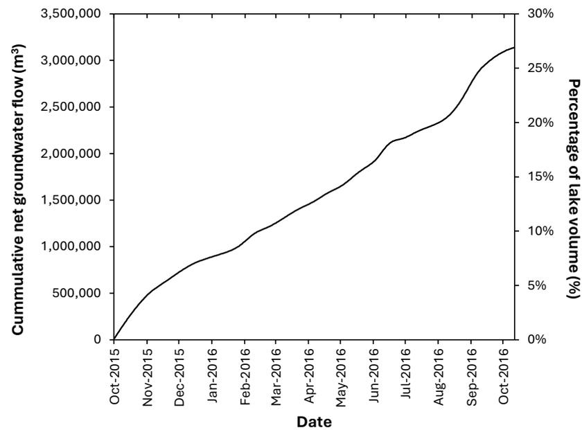
**Figure 8.** Time series of cumulative net groundwater flow in both total cubic meters ( $\text{m}^3$ ) and percent (%) of average lake volume. A total of 26.3% of the average lake volume entered the lake via groundwater net flow over the course of data collection.
