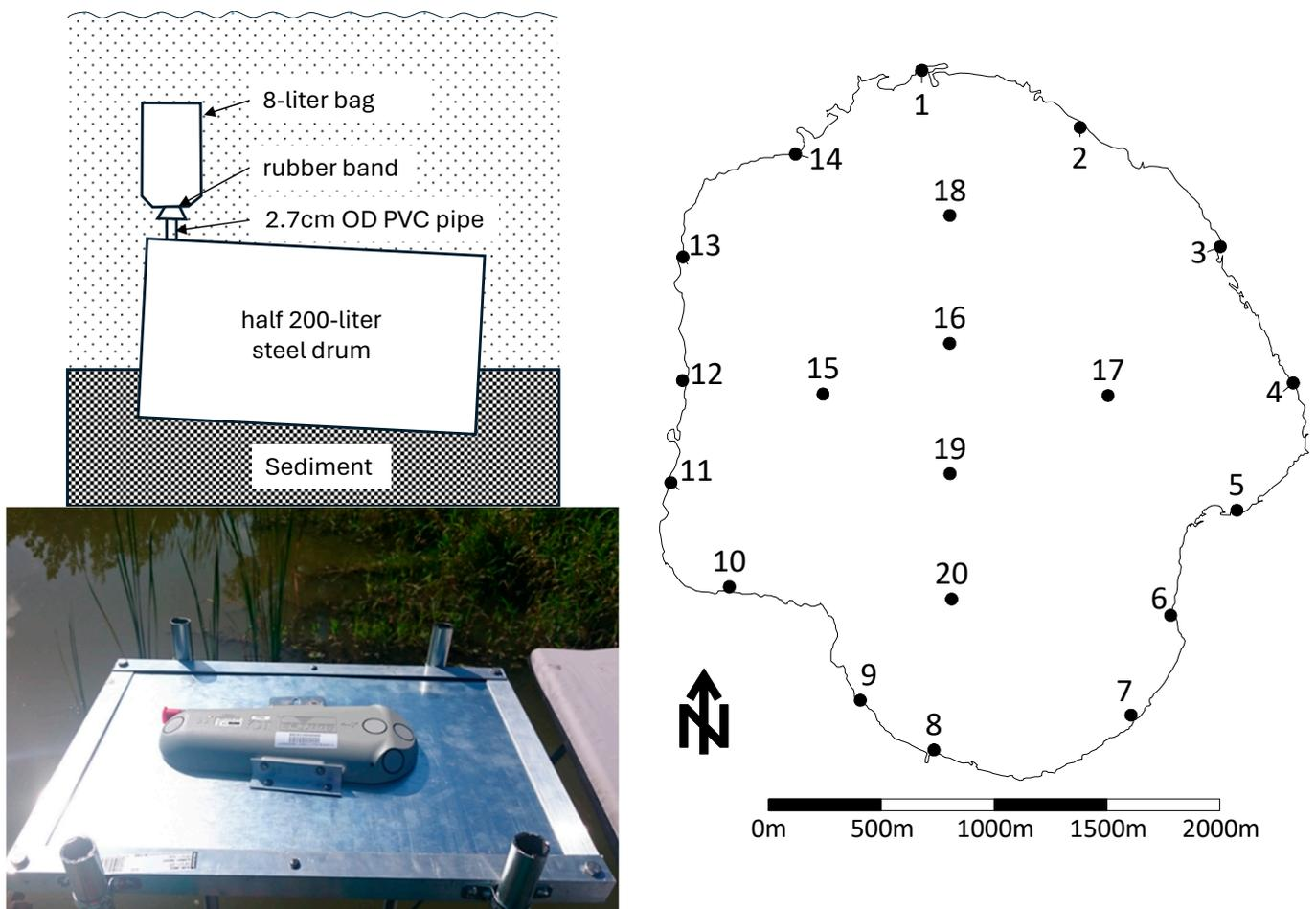
**Figure 3.** (Top Left) Diagram of the slightly tilted groundwater seepage meter with its collecting bag attached. (Bottom Left) Sontek IQ flow velocimeter for canal water flow measurement. (Right) Location of the seepage meters (closed dots) within Lake Trafford. Meters 3, 5, 10, and 13 were used to estimate the seepage variation for a given location.
