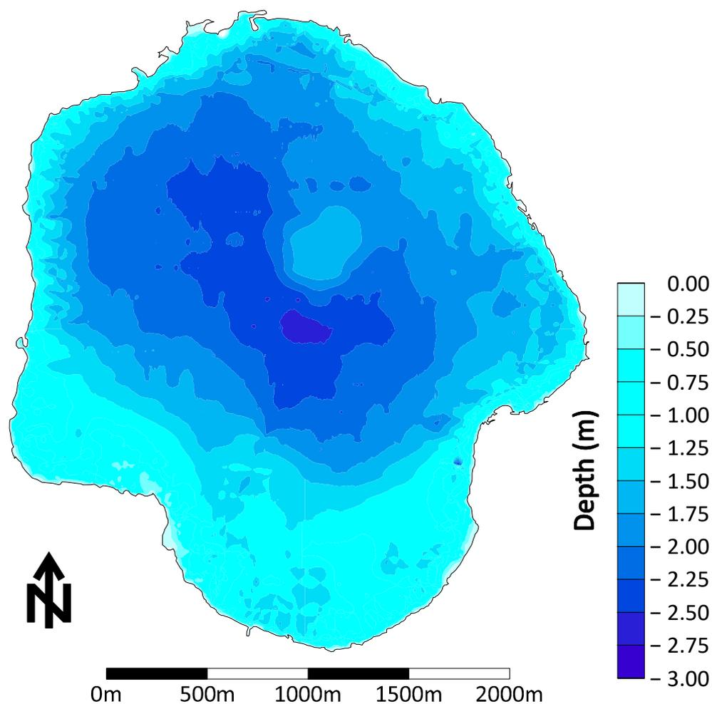
**Figure 4.** Bathymetric map of Lake Trafford for a surface water elevation of NAVD'88 5.53m. Bathymetry data were used to determine volumes and planar surface areas at various lake levels using Surfer 27.
