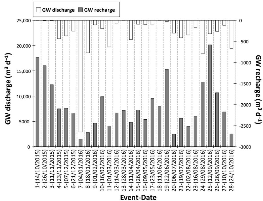
Figure 6. Total groundwater discharge (gray bars) and recharge (white bars) in m<sup>3</sup> d<sup>-1</sup> for each sampling event 1 through 28 (associated dates in parentheses).
