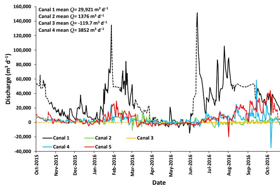
**Figure 9.** Hydrographs of each of the canal discharges ( $Q$ ,  $\text{m}^3 \text{ d}^{-1}$ ) from 1 October 2015 to 24 October 2016. Mean daily  $Q$  is also reported for comparisons. Estimated portions of the hydrographs appear as dashed lines (cf. text for more information).
