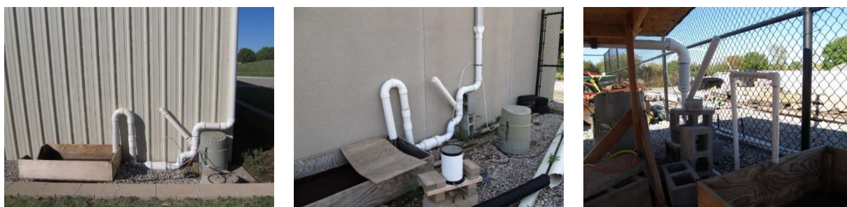
Figure 1. Modified downspout configuration for the metal roof (left), tar and gravel roof (middle), and asphalt shingle roof (right).
