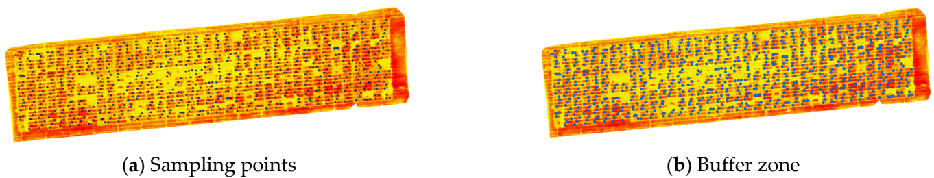
Figure 8. Plant height (CHM) extraction sampling points and buffer zone. Panel (a) shows the distribution of sampling points across the cotton field, where plant heights are extracted from CHM data. Panel (b) illustrates the established 30 cm buffer zones around each sampling point, used to accurately match canopy height values from geographic coordinate data within the ArcMap software.
