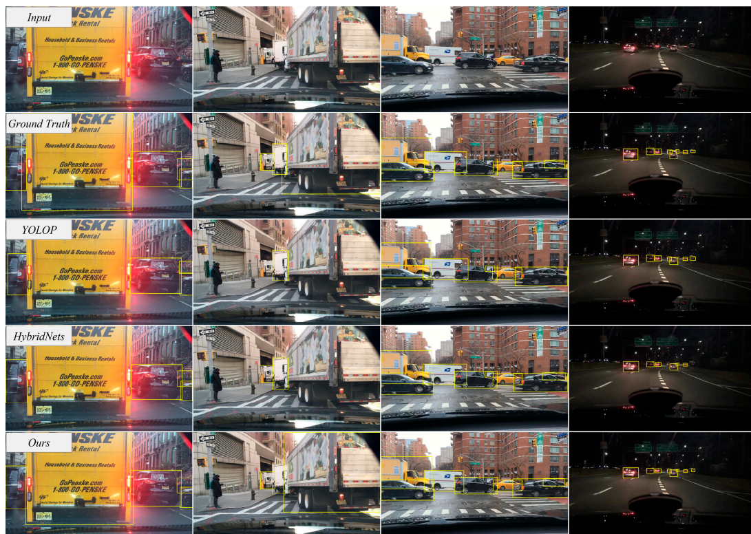
Figure 5. The comparison chart of traffic object detection. The rows from top to bottom are the input images, the ground truth, and the predictions of YOLOP, HybridNets and ours, respectively. The yellow boxes indicate the traffic objects.
