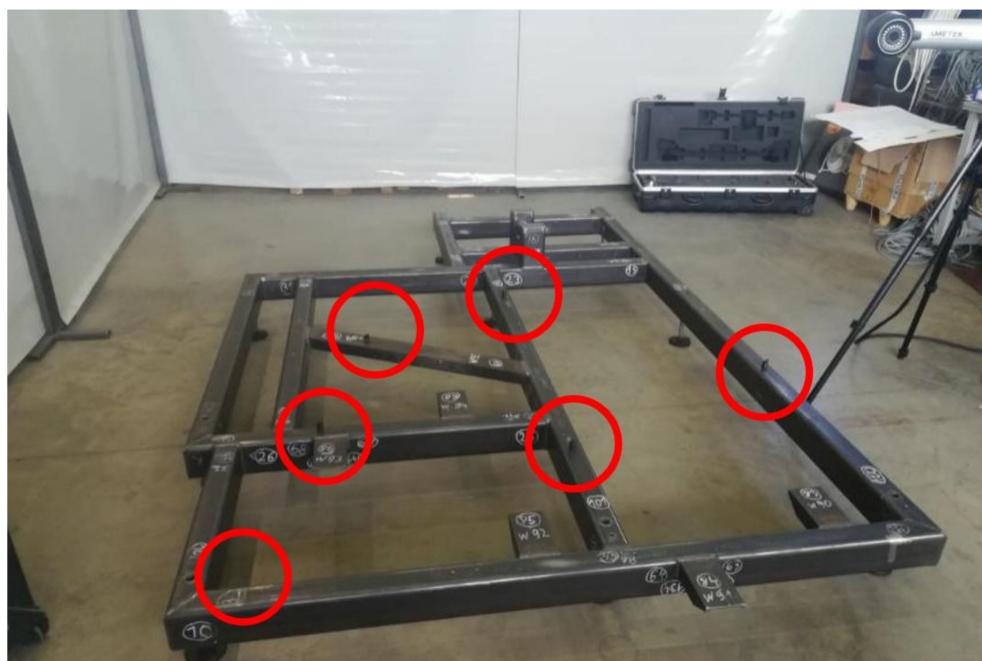
Figure 5. Example of the location of reference points on the tested frame No. 1.
