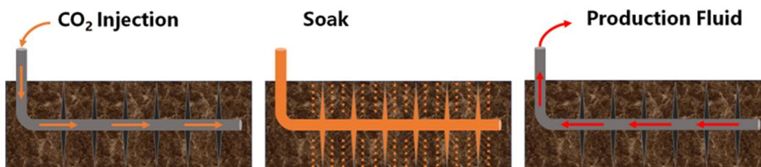
**Figure 1.** CO<sub>2</sub> huff-n-puff in multi-stage fractured horizontal well.
