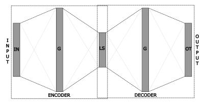
Figure 4. The encoded values are concatenated, forming a single latent space.
