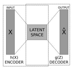
Figure 1. High -level representation of an auto-encoder.
