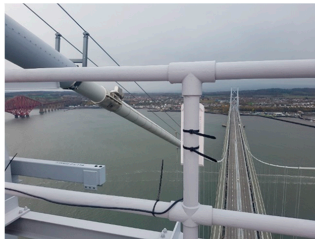
Figure 4. A TP-Link Wi-Fi transceiver point (CPE510) installed atop the northeast tower of the Forth Road Bridge.
