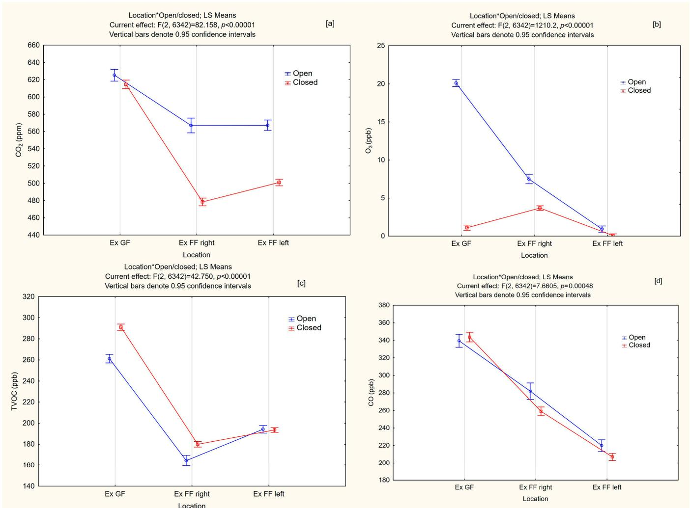
**Figure 4.** The factorial ANOVA results (the interaction effect Location\*Open/closed) for the air pollutant concentrations (CO<sub>2</sub> [a], O<sub>3</sub> [b], TVOC [c] and CO [d]) in exhibition halls.
