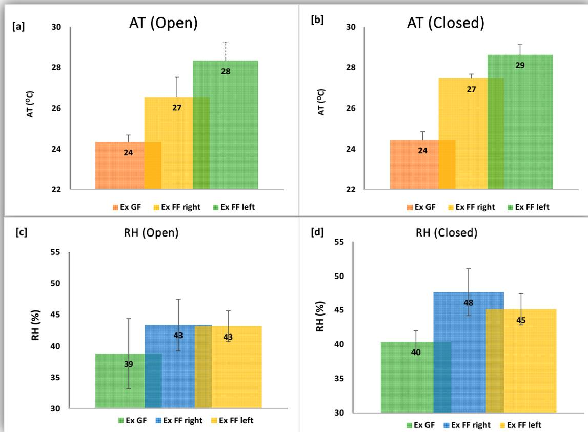
**Figure 3.** Comparison of mean ( $\pm$ SD) AT ([a,b]) and RH ([c,d]) between open/closed conditions in exhibitions at the Abdera museum.
